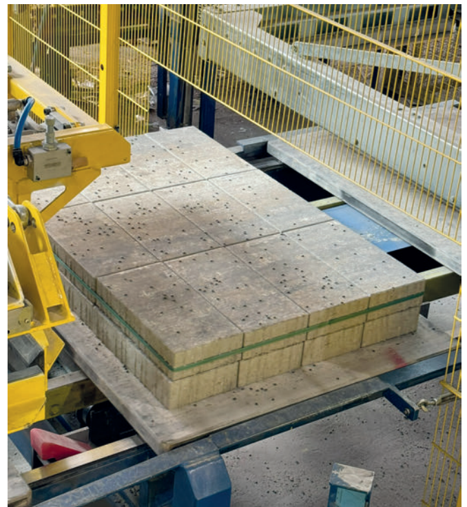
Fig. 4: The Kuka KR 700 palletising robot has a lifting capacity of 700 kg, equivalent to a load of 350 kg of concrete products.
