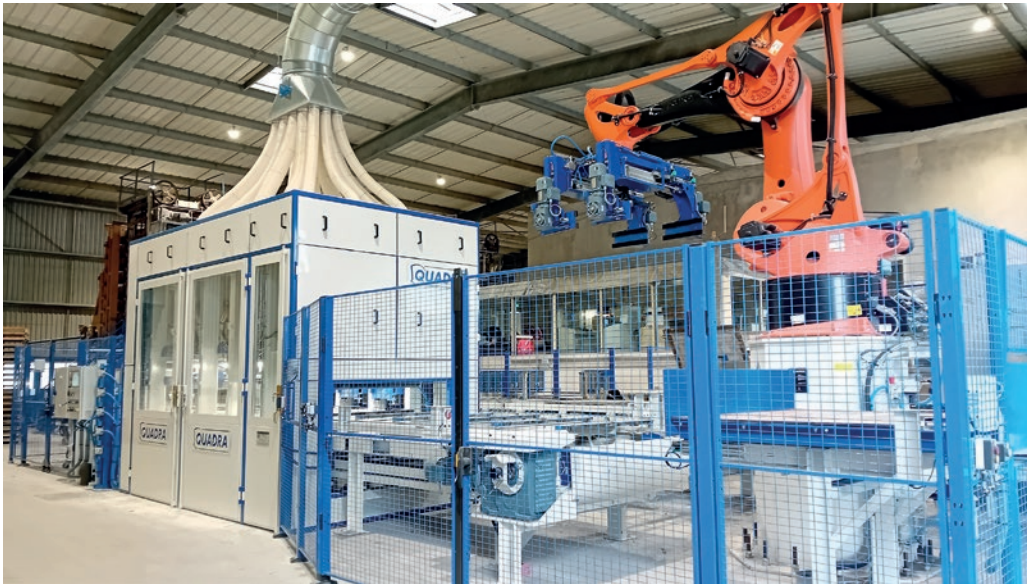
Palletising robot at the grinding machine conveyor to cub the grinded blocks.
