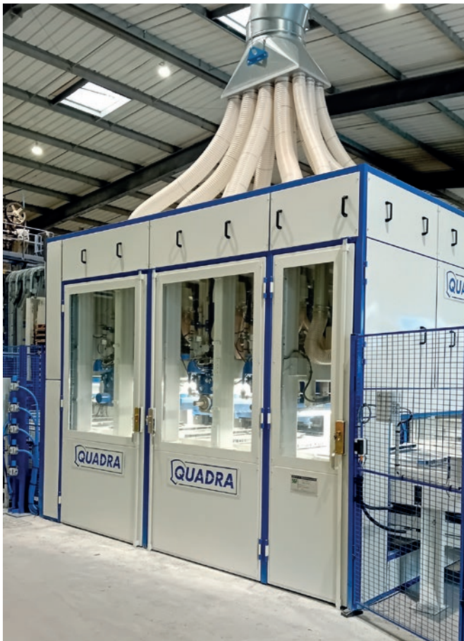
Quadra grinding machine: protected by an independent soundproof cover, designed to reduce noise and facilitate access.
