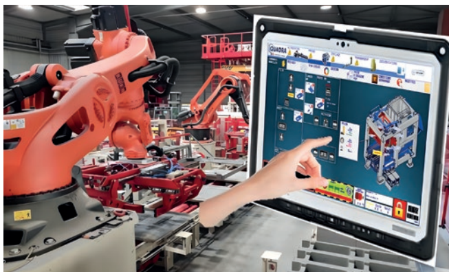
WiFi-connected touchscreen tablets to adjust settings directly in front of the machine.
