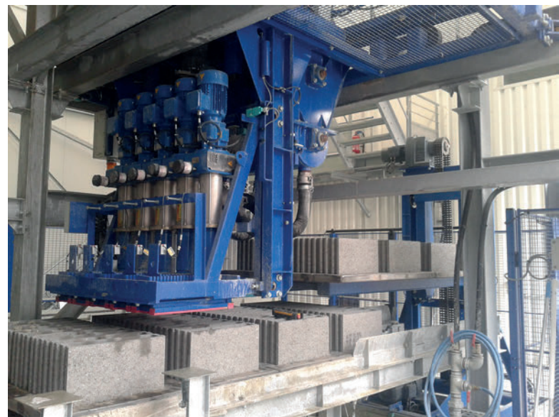
Air'Mousse dosing and filling unit
