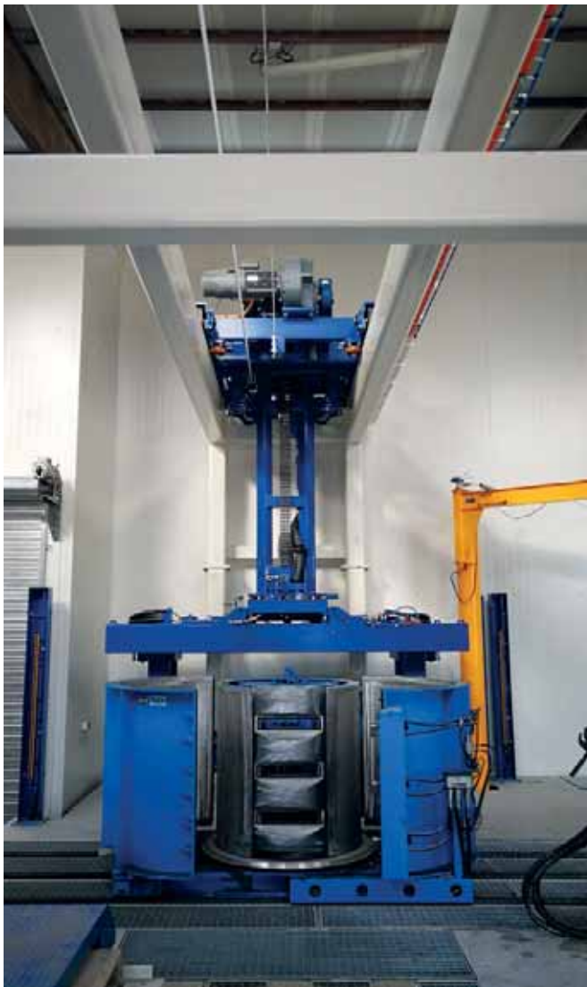
For manhole risers and cones, the mold is open before demolding.
