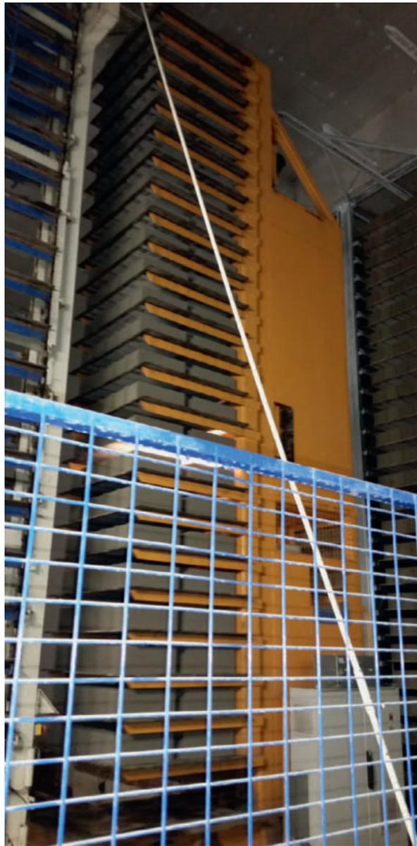
The curing area provides capacity for 4,896 pallets and is equipped with a ventilated, humidity-controlled system
