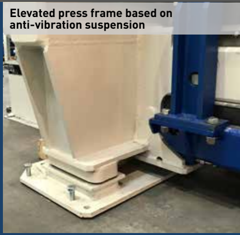
Vibration with modular strength and adjustable frequency patented
