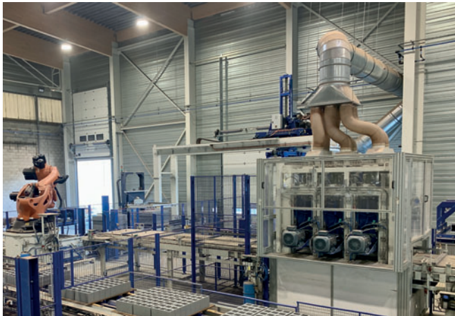
Grinding machine located between the lowerator and the palletization area.
