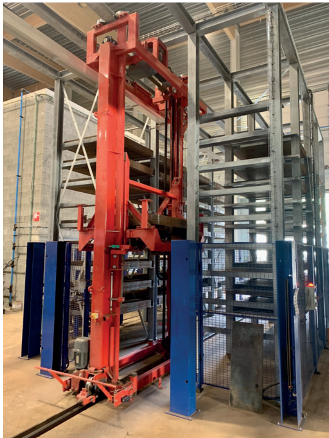
A storage of 860 pallets managed automatically by a storage and retrieval machine ensures continuous operation of the production unit.
