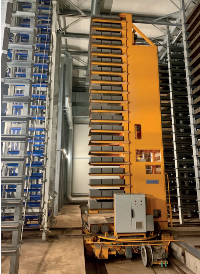
A finger car with rotative platform, carrying 20 pallets, performs storage and retrieval operations. The curing area has a 4,920 pallets capacity and is equipped with a ventilation system.
