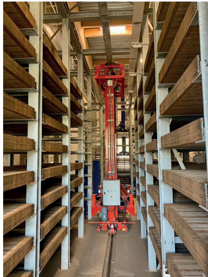
A storage of 860 pallets managed automatically by a storage and retrieval machine ensures continuous operation of the production unit.
