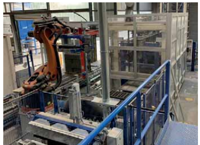
The robot is controlled with a software that is integrated within Quadra's interface. The recipe settings are easily adjustable from the control desk.
