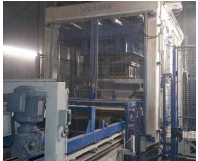
Vibrating press type Quadra 5.
