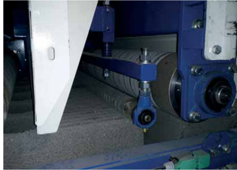
This grinding machine type "diamond rolls" was perfectly adapted to the production of Pomel Beton.
