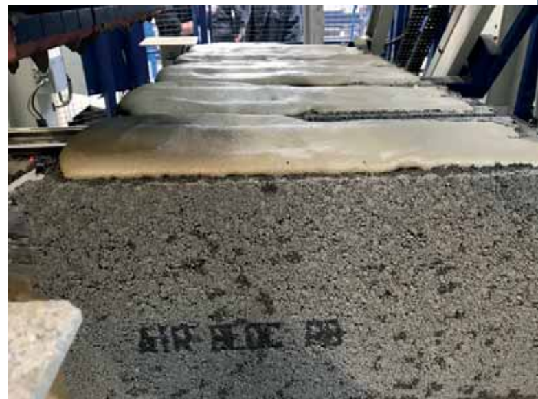
Manufacture of the insulating block "Air'Bloc".
