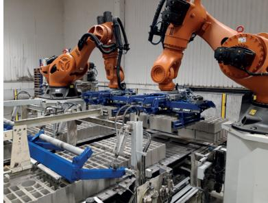
This new cubing line consists of three robots operating simultaneously, following the cycle time of the vibrating press, within operating condition combining precision, speed, flexibility, and reliability.
