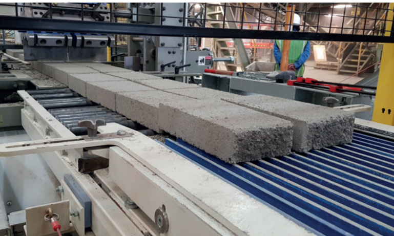
Splitting waste is removed by a waste conveyor belt
