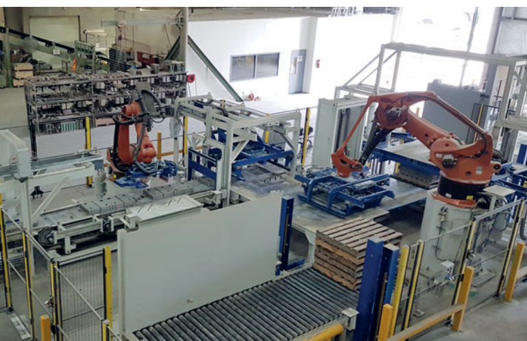
Kuka KR240 6-axis robot for pattern making and KR700 4-axis palletizing robot
