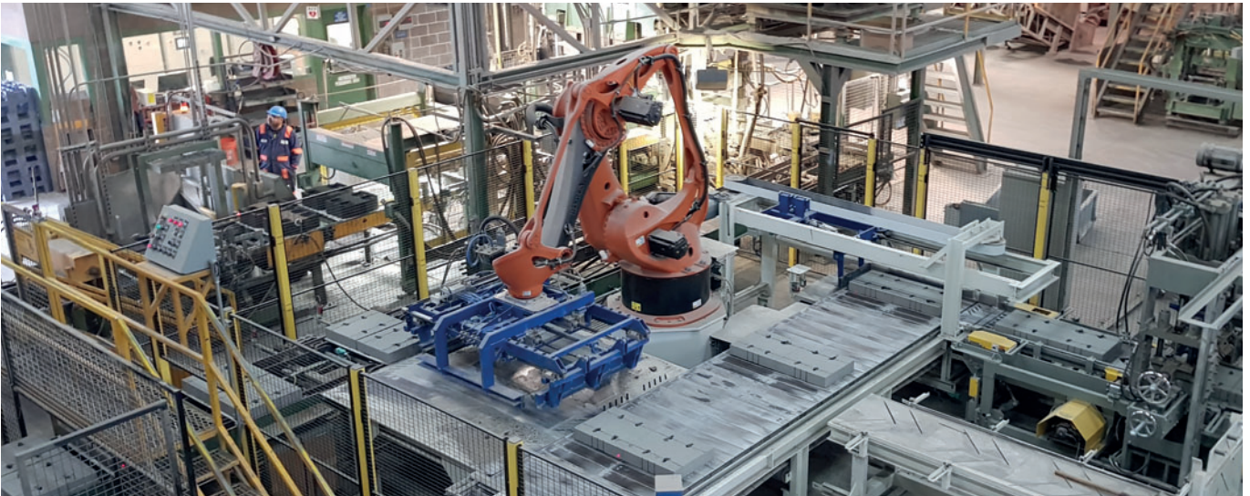
Depalleting robot Kuka KR700 4-axis, with pneumatic clamp designed and manufactured by Quadra
