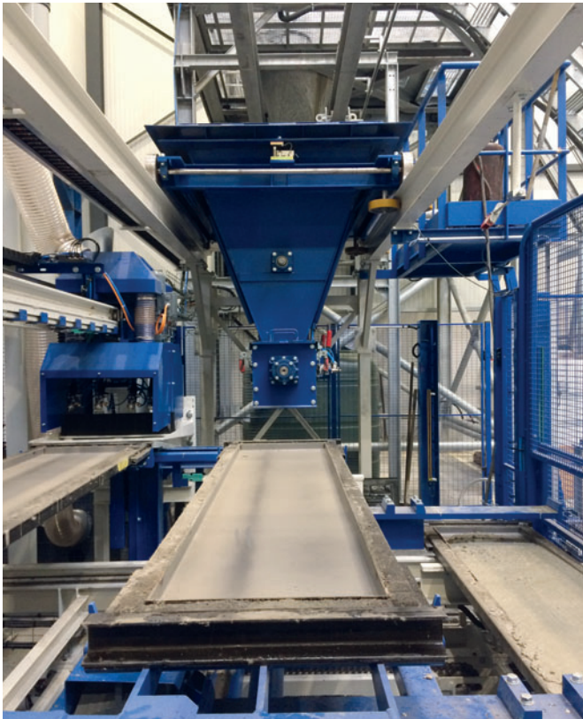
Automatic mould filling and dosing system
