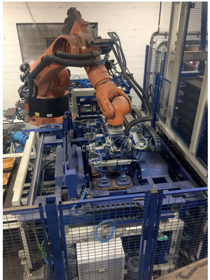
6-axis robot type Kuka KR360, driven by PLC.
