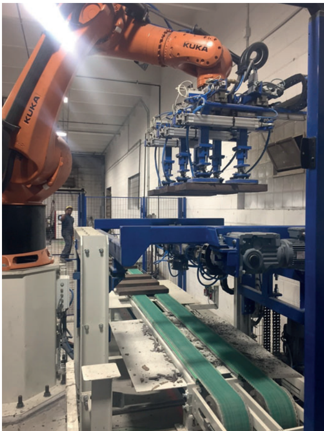
Belt conveying system & product turning device
