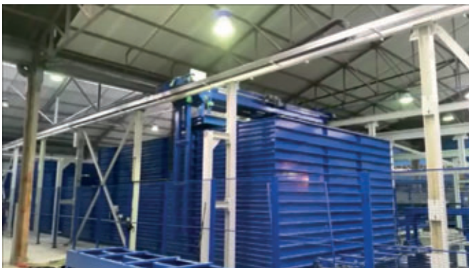
The curing area may receive up to 210 demoulding pallets dimensioned 5,450 x 1,250 x 220 mm.
