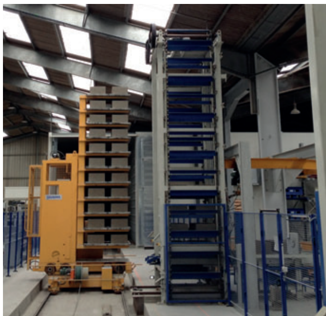
The finger car can handle up to 22 pallets at the same time.
