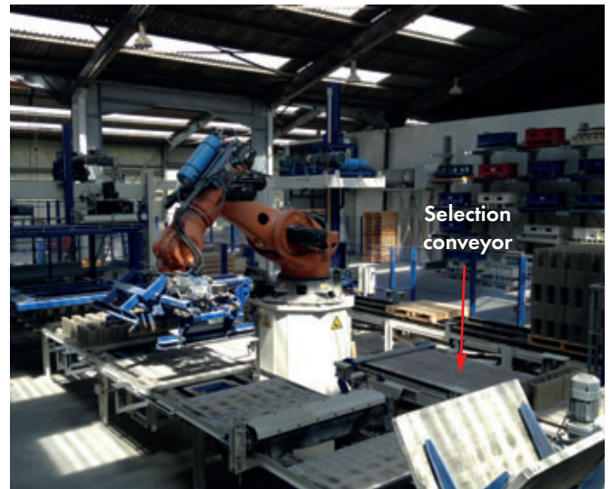
Featuring 6 axes, the cubing robot Kuka KR 1000 can handle 1,000 kg.
