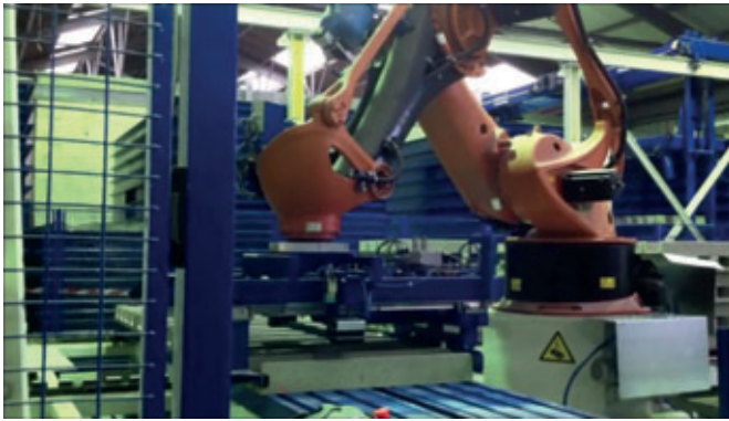
The palletizing station is equipped with a Kuka PA 700 robot.
