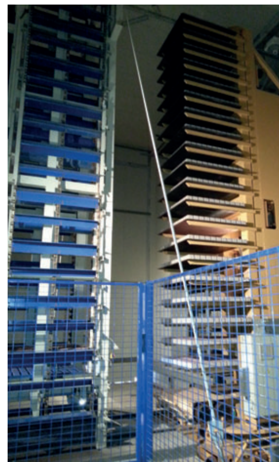
Finger car unit for 20 production boards
