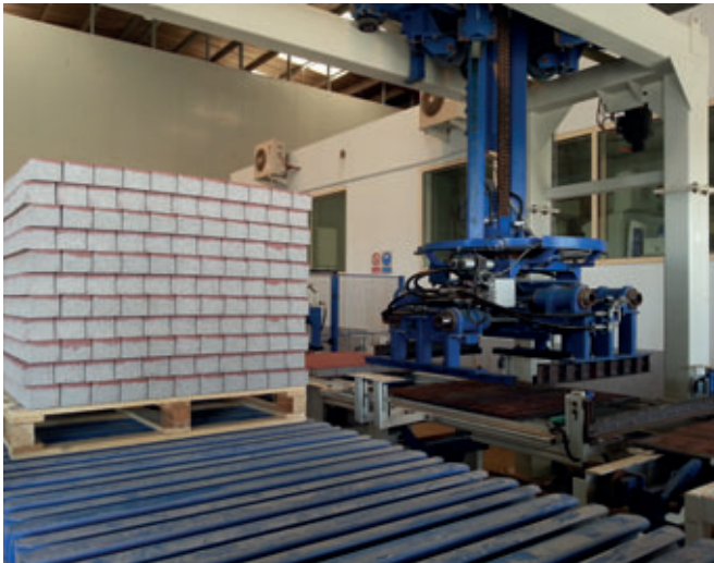
Removal of the finished cubes on pallets
