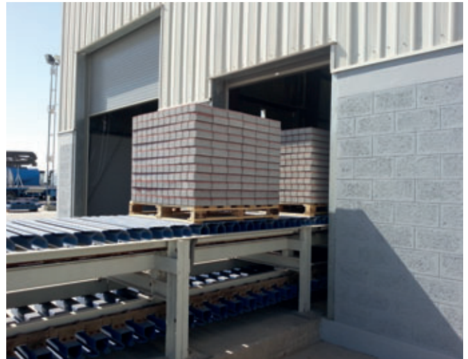
Exit of dry products via slat conveyor
