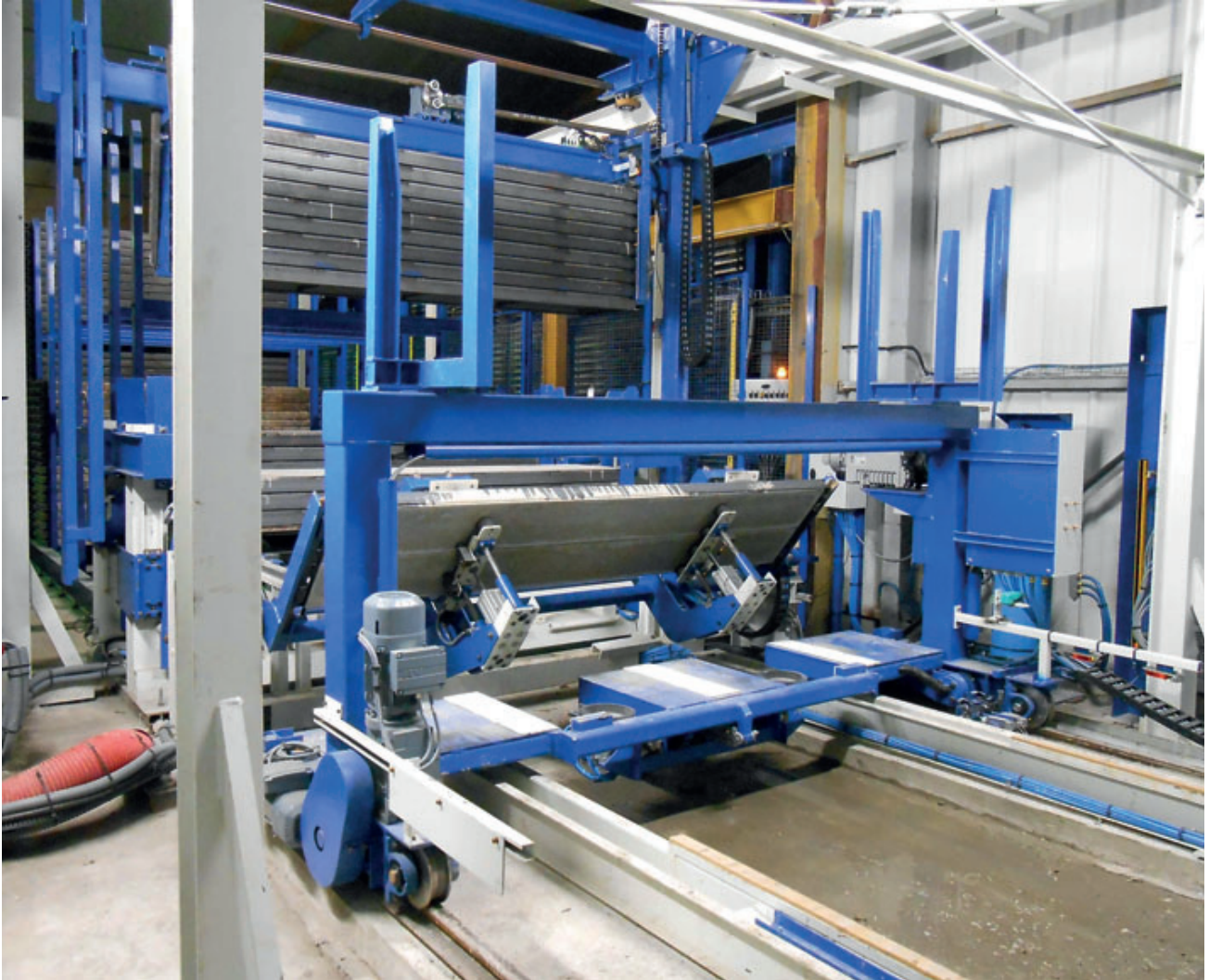
Demolding by turning (180°)
