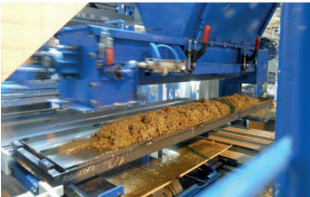
Concrete feeding: Automatic mold dosing and mold filling
