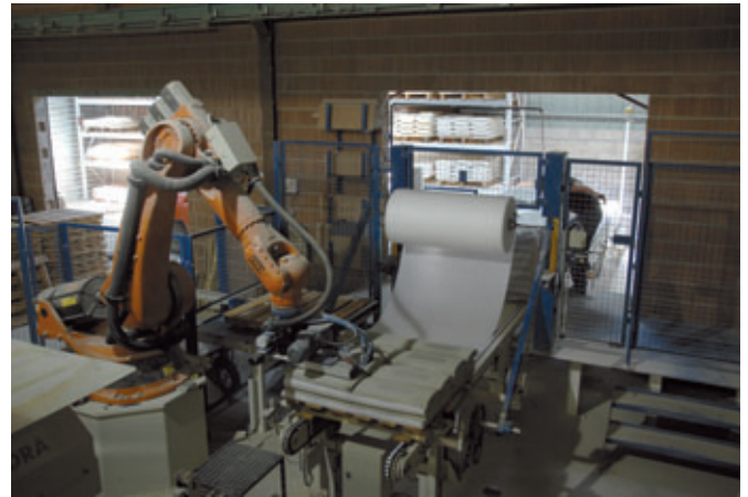
The 6-axis articulated robot palletises the products using a vacuum clamp
