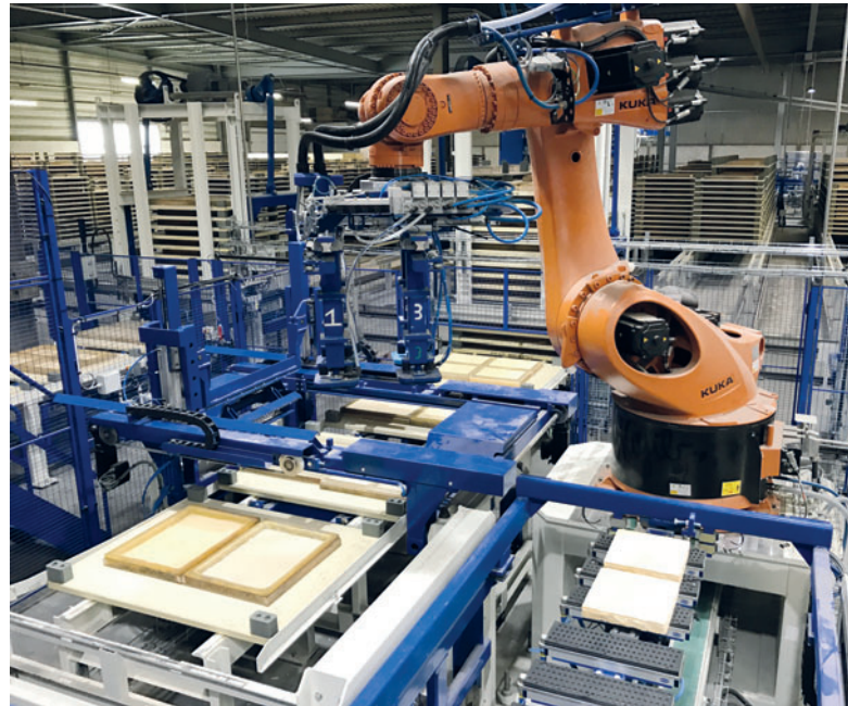
The demoulding operation is performed by a 6-axis robot type Kuka KR360, allowing the demoulding of products weighing up to 120 kg
