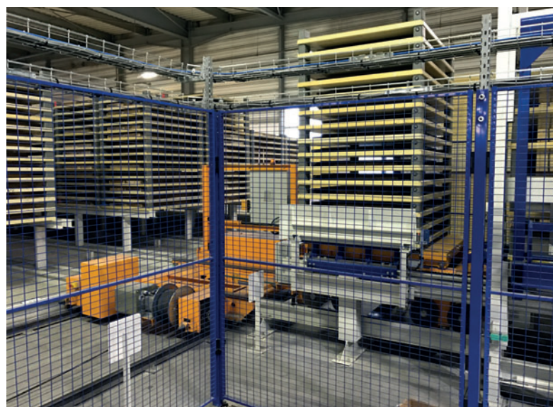
The curing area can store up to 5200 pallets
