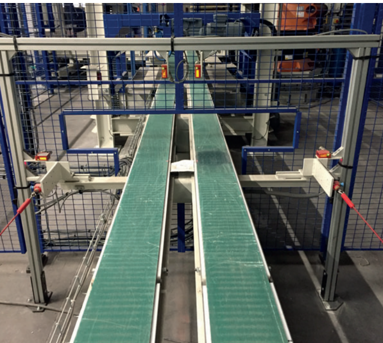
The palletizing system is equipped with a measuring system including lasers and sensors: view of the quality checking station
