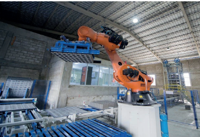
The state-of-the art 6-axis robotic cuber with a payload of 1300 kg. This robot is able to form cubes by using blocks instead of wooden pallets
