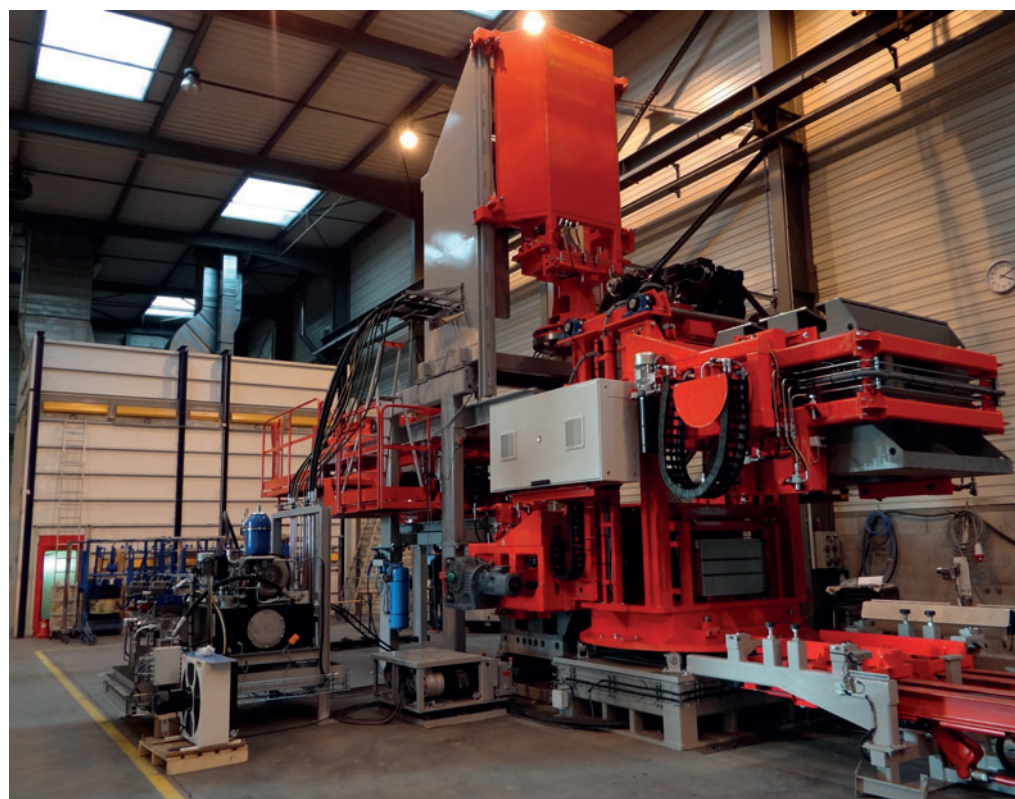
Fig. 3: Vibrating press with semi-dry demoulding by turning over
