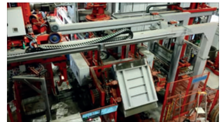
Fig. 5: Gantry for handling demoulding pallets
