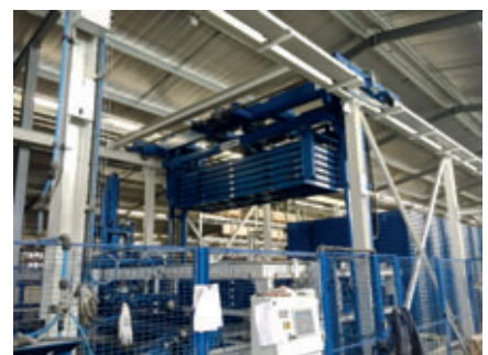
Automated mould storage
