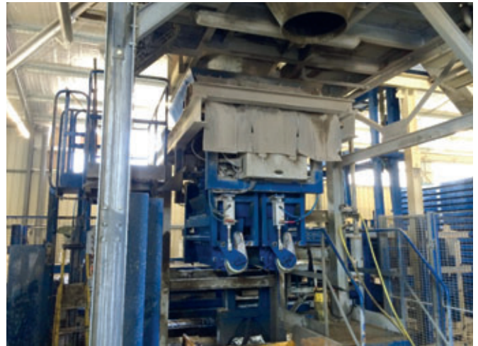
Automatic mould filling system
