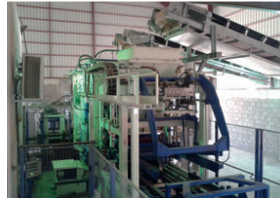
The block machine Q12 HP displays a striking industrial rate: between 13 and 15 seconds for manufacturing two-layers paving stone.
