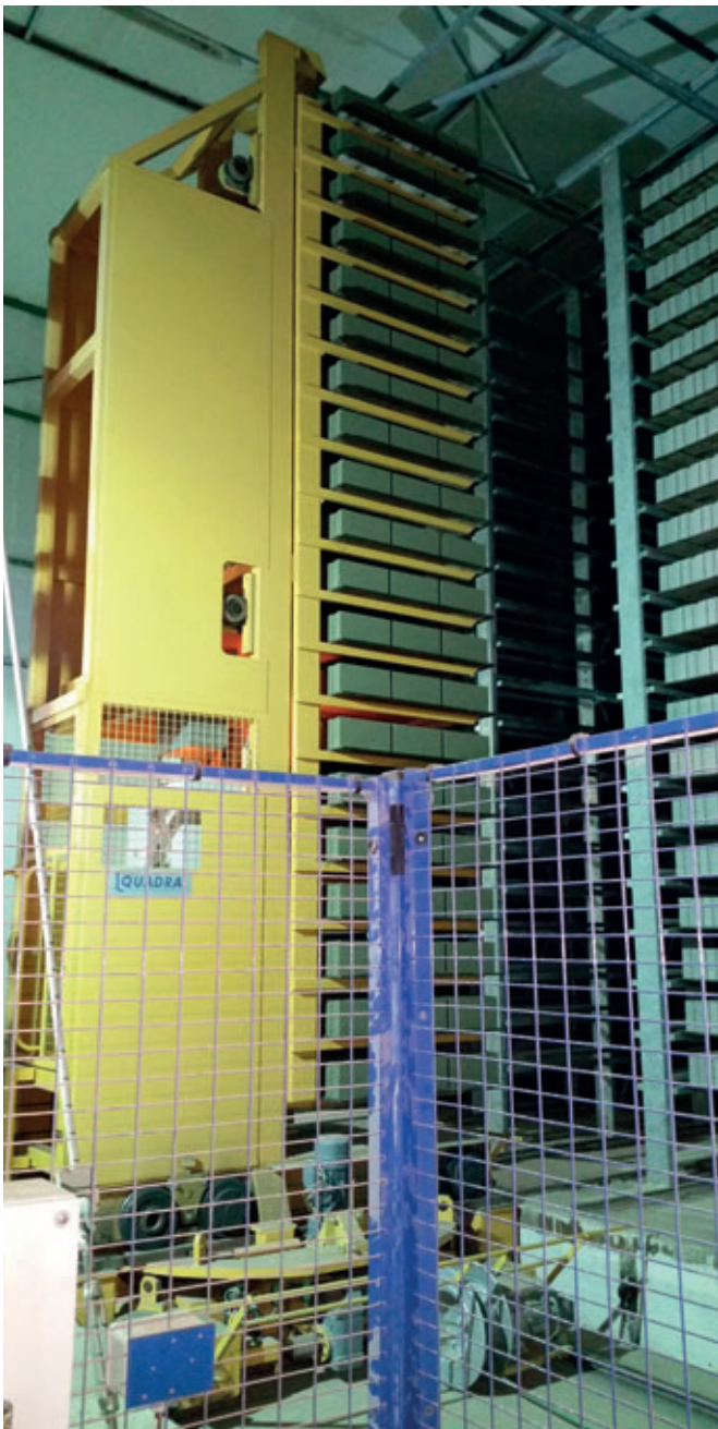
The finger car with rotating platform performs the storage operations.
