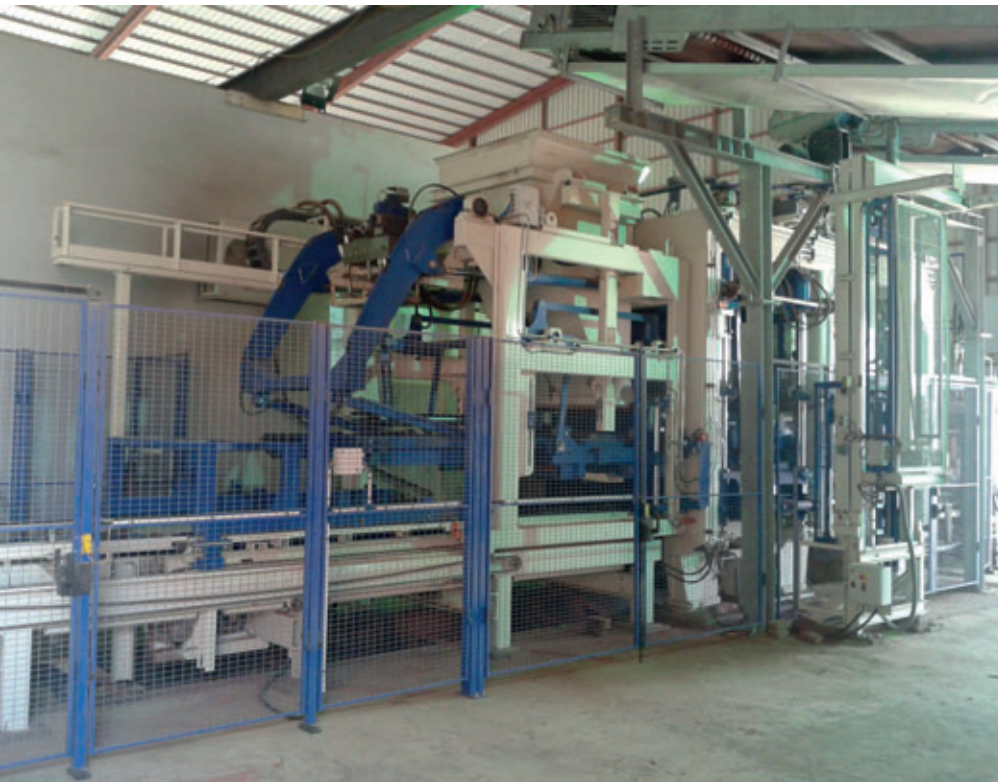
The block machine Q12 HP displays a striking industrial rate: between 13 and 15 seconds for manufacturing two-layers paving stone.
