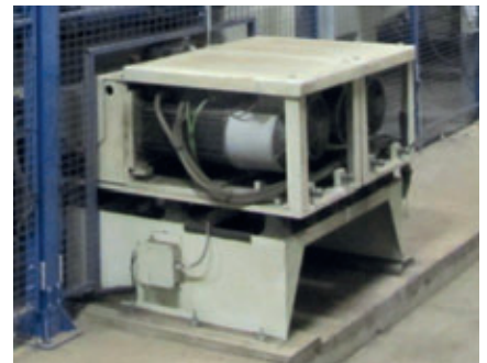
The vibration motors are located on one side of the block machine allowing direct access.
