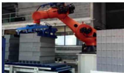
3) The lower rank of the pallet is formed from the product settled in the «virtual» pallet.
