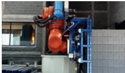
2) The robot is retrieving one row for creating the low rank of the product pallet.
