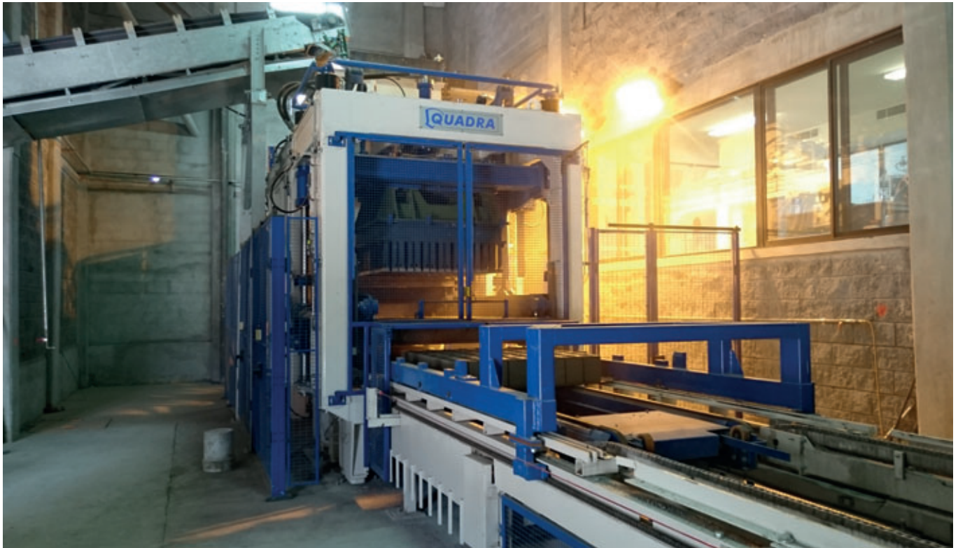
Block-machine type Q12 HP: rugged and ventilated architecture that allows high-quality product manufacturing within high rates.
