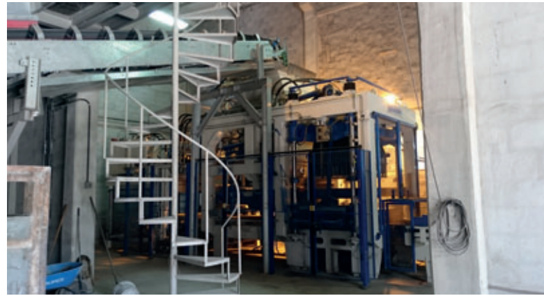
Rational configuration: frame (massive and heavy one-piece steel structure) based on anti-vibration feet. Optimal filling and vibrating system: patented process
