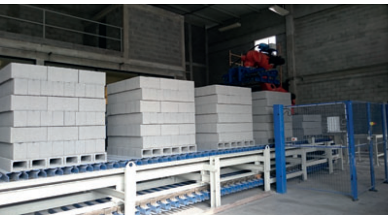
Cubing robot type Kuka KR 1000 equipped with 6 axes: maximal load of 1300 kg
