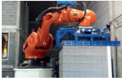
1) The robot is cubing the «virtual» product pallet.
