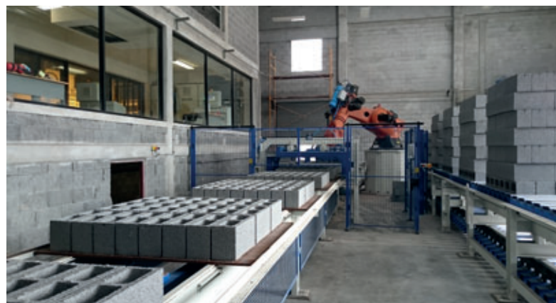
Following the curing and the transfer to the lowerator, the pallets loaded with products are finally transferred to the cubing station via a walking beam conveyor. This type of conveyor lifts and moves the pallets without any friction. It also means no wear, and no noise.
