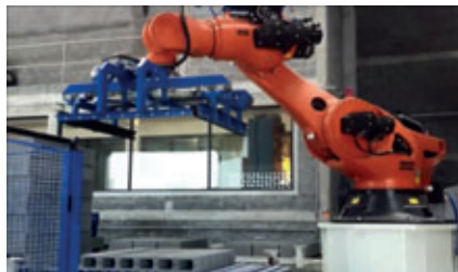
3) The lower rank of the pallet is formed from the product settled in the «virtual» pallet.
