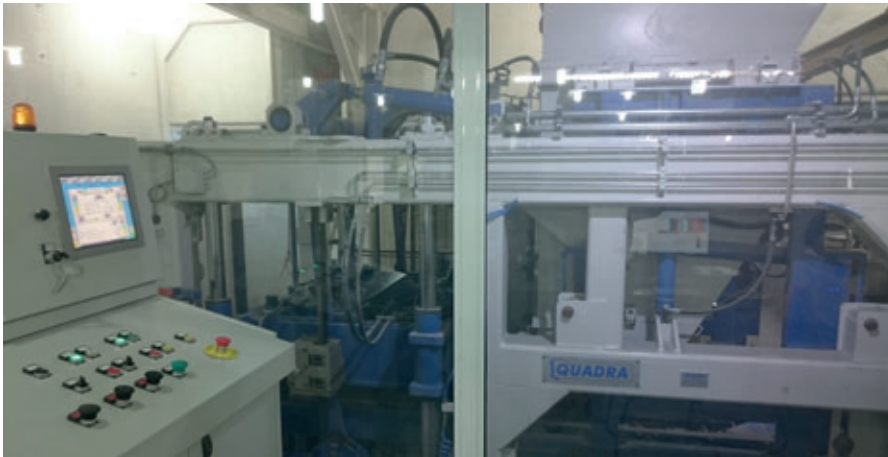
Equipped with glazed windows, it enables the operator to control the block-machine while watching the overall plant.
