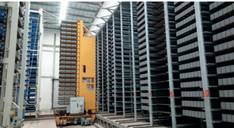
The finger car with rotating platform: The curing solution is engineered to give the optimal utilisation of space
