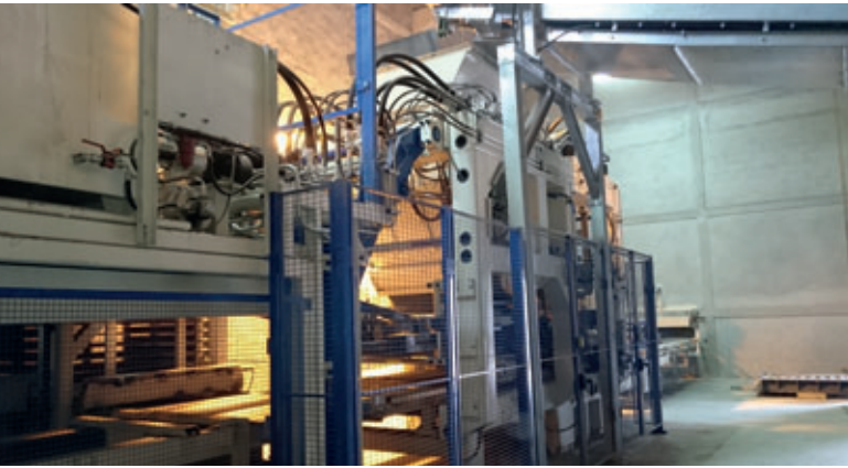
Rational configuration: frame (massive and heavy one-piece steel structure) based on anti-vibration feet. Optimal filling and vibrating system: patented process
