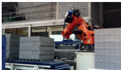
4) The robot is making the product pallet from the product on the production boards.
