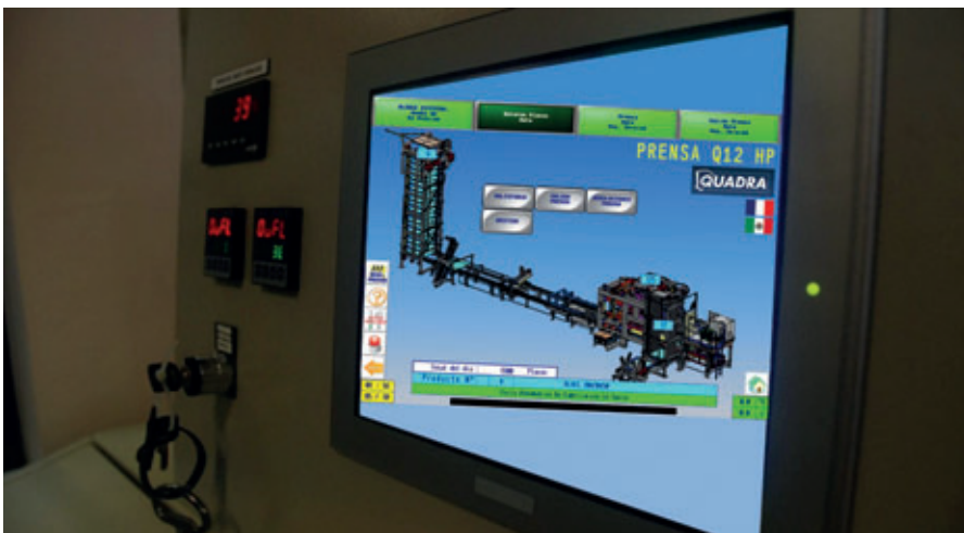
Clear, intuitive and user-friendly interface allows easy modification of the block machine settings
