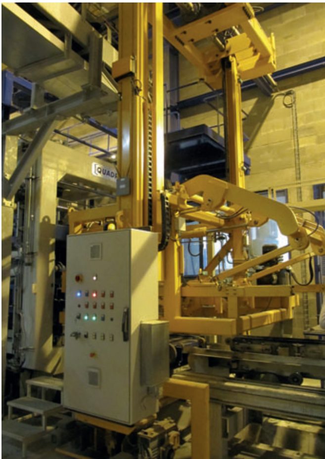
Production changeover operated by the stacker crane
