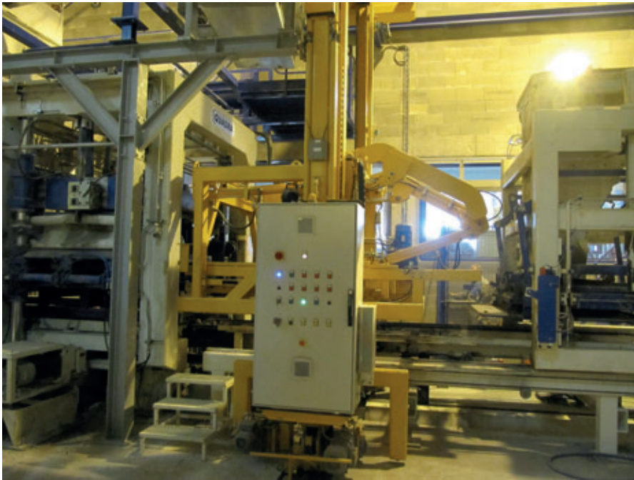
Stacker crane ready to incorporate the new mould
