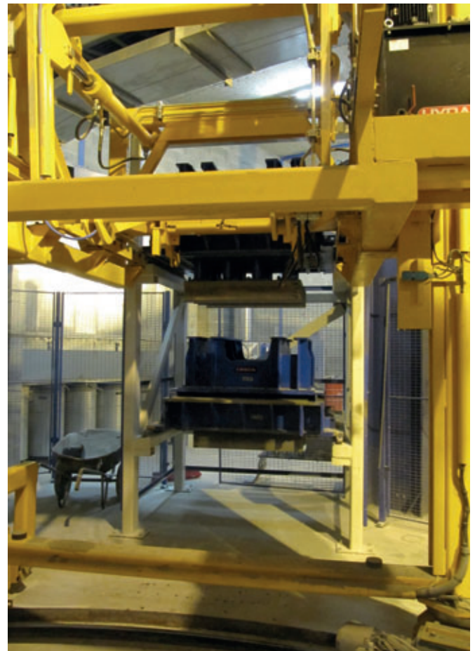
Rack close to the block machine
